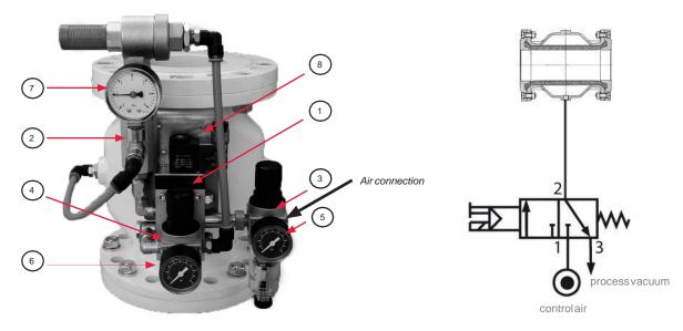
The AKOVAC Comfort model allows for the specific setting of separate pressures on the control unit for the control pressure for closing the pinch valve (by turning the pressure regulator (4), pressure monitoring by the manometer of the pressure regulator (6)) and the control pressure which regulates the level of vacuum (by turning the filter regulator (3), vacuum monitoring by the manometer (7)).
