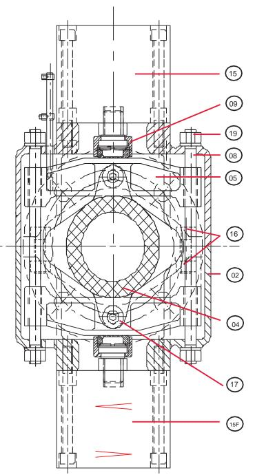
**PA2: DN 65 - 200mm,** with two single acting cylinders. The valve is spring closed.
