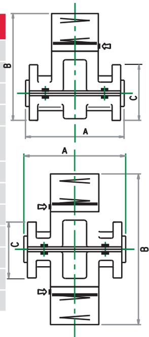
\* = Flange connection: TK= pitch circle / d = bolt holes
